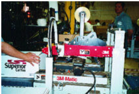
The filled corrugated cases are fed into the case-sealing machine.
